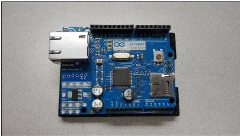
When you have obtained the shield, attach it to the top of your Arduino. Now, you can open the Arduino IDE, and the first example you'll use is a simple web page access of data. To do this, open the **WebServer** example by navigating to **File | Examples | Ethernet | WebServer**, as shown in the following screenshot:
